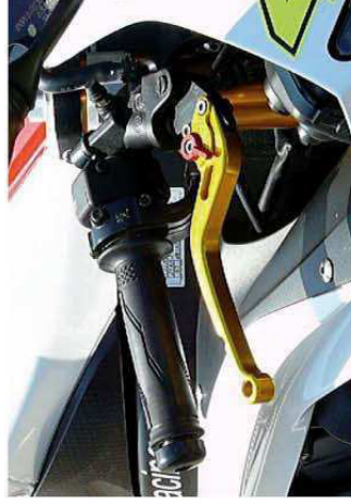
6) TITAX lever on the motorcycle. Check function and position of the brake lever adjustment. Check function of brake performance
