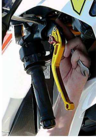
5) Take care of the brake light switch during mounting (if any) Use a tool spanner and screwdriver to mount back nut and screw which hold the lever. Use 8-10 Nm torque when tightened the screws also use manufacturer manual bike specification for confirmation. Check function of brake light switch find the right position of the brake lever adjustment. The lever has to be caught by the first 1/3 of your fingers than it is mounted and adjusted correctly
