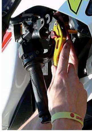
4) Lube the lever bearing before mounting. Use only certified lubes for bearings. Put TITAX lever back instead of original lever.
