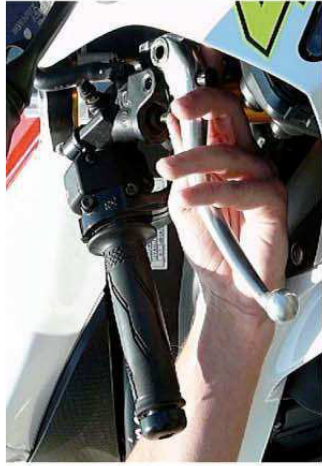
3) Take out the screw and nut and move original lever out.
