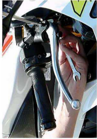
2) Use a tool spanner and screwdriver to release nut and screw which hold the lever. Use the size of spanner according to the size of nut.
